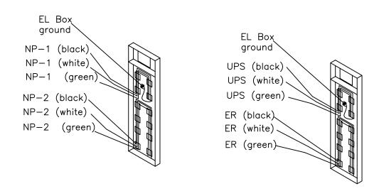
Each upright per side can be configured with one 12 outlet 20 amp electrical box with data. Electrical box can accommodate 1,2, or 3 circuits of power per service and several different types of power, i.e. ER, UPS, normal power, 220V and GFI where applicable. Data is isolated from electrical wires at all times. ER and UPS service comes with an independent ground and neutral wire
