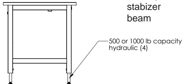
tubular FRAME 2 X 2 X 16ga BOX tube, SIZES
